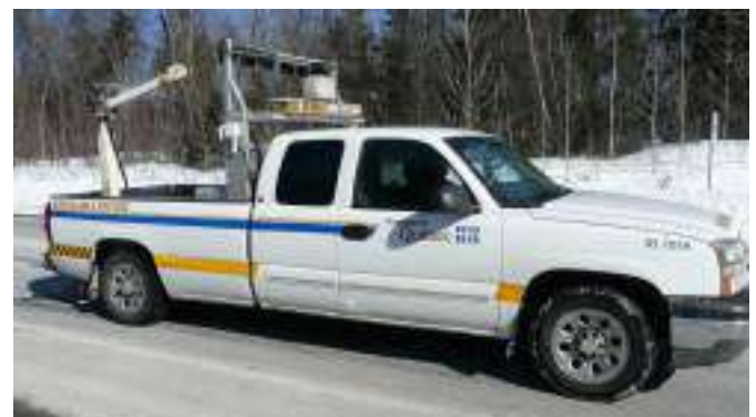
Figure 4 – Mobile road weather station
