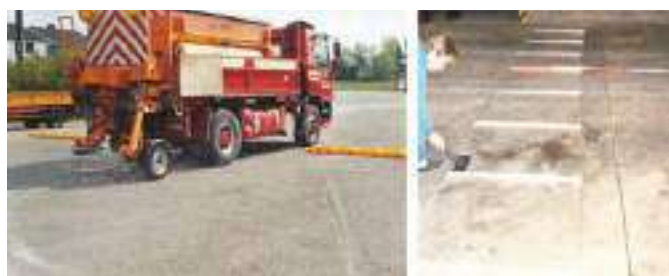
Overview of the initial technical inspection of spreaders (for wet (left) and dry (right) salt spreading) – Walloon region
