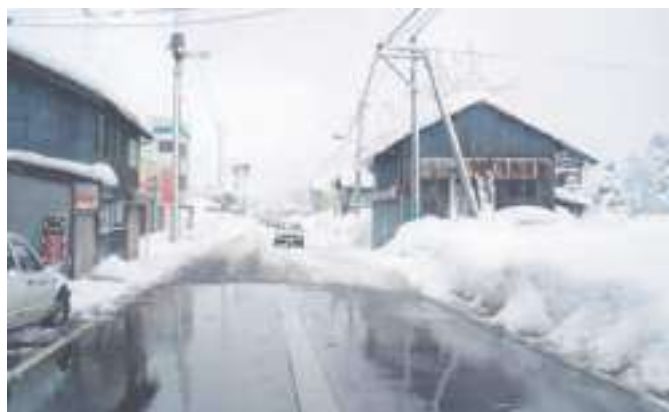
Figure 12 - Effect of snow-melting sprinkler
