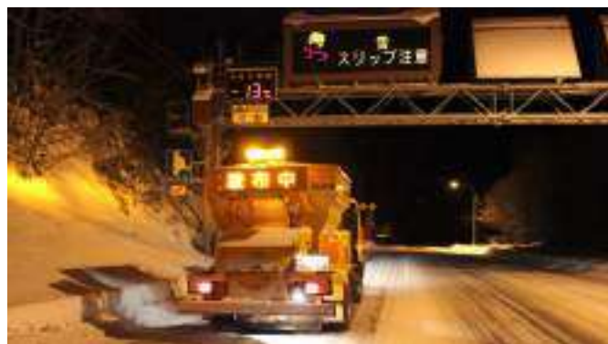
Figure 8 - Application of anti-freezing agents
