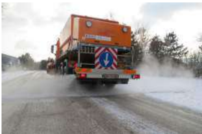
Figure 5 – Truck with brine spraying device
